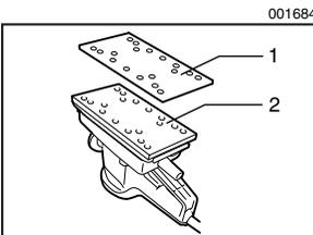
1. Hook-and-loop type of abrasive paper with pre-punched holes
