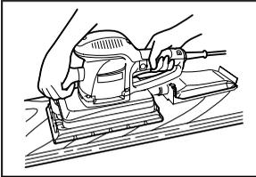
Turn the tool on and wait until it attains full speed. Then gently place the tool on the workpiece surface. Keep the base flush with the workpiece and apply a light pressure on the tool.
