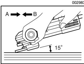
ALWAYS hold the tool firmly with one hand on housing and the other on the side handle. Turn the tool on and then apply the wheel or disc to the workpiece.
